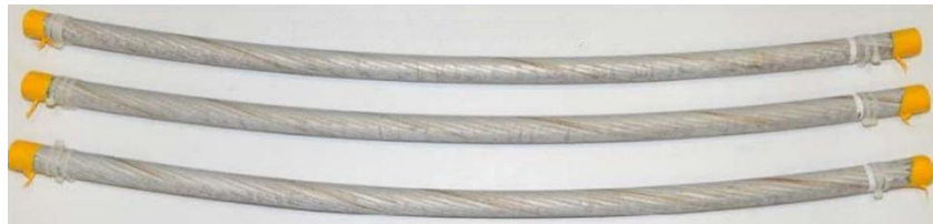
Figure-9 550 mm 2 ACFR/TW Conductor specimens of salt spray test
